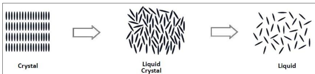
Fig 1: Formation of liquid crystal phase between crystal and liquid state of aggregation
