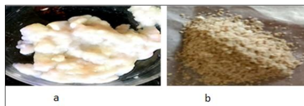
Fig 1: In the extraction of tamarind seed gum a) Precipitated mass and b) tamarind seed gum powder.
