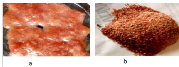
Fig 2: In the extraction of moringa gum a) Precipitated mass and b) moringa mucilage powder.
