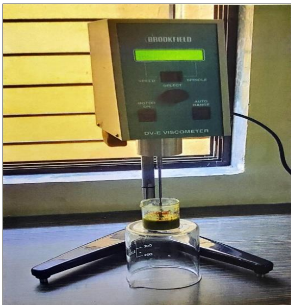
Fig 1: Viscosity determination by Brookfield Viscometer
