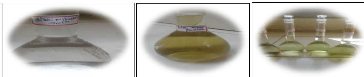
Fig 8: Photograph of biosynthesis of Silver Nanoparticles from Punica grantum extract A) Before synthesis, B) After 15 min & C) After 24 hrs.
